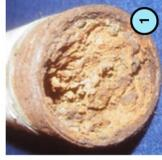
PROBLEM: GALVANIZED IRON WATER SUPPLY PIPES ARE CORRODED
